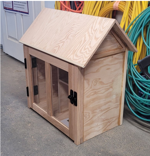
Pikes Peak Habitat volunteer Bruce Latimer built the little library (above, before installation and finish) with marine-grade plywood supplied by Pikes Peak Habitat. He researched and purchased weatherproof fixtures himself. Below, he inspects the clasp on the completed library.
